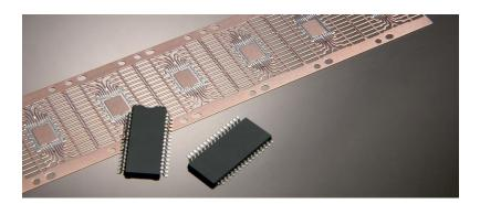
**SOIC** The Small Outline Integrated Circuit is available in a number of variations, including SOP (Small Outline Package), SSOP (Shrink Small Outline Package), SOJ (Small Outline J-Leaded), TSOP (Thin Small Outline Package), and TSSOP (Thin Shrink Small Outline Package). The SOIC package is desirable for its small footprint on the circuit board. SO lead frames are available in single-pad, dual-pad and matrix designs.
