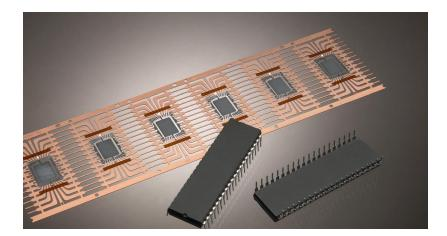
PDIP/SPDIP The Plastic Dual In-line Package/Shrink Plastic Dual In-line Package has a rectangular plastic body with two rows of leads that are bent up from the package body at a slight angle. Its most common use is through-hole insertion mounting in applications such as logic, processor and memory devices. QPL also delivers IDF (Interdigitated Frame) versions that enable more lead frames to be oriented along a strip, resulting in increased throughput in assembly.
