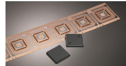
PLCC The Plastic Leaded Chip Carrier has leads on all four sides with J-shaped bends and is available with a variety of pad designs, such as dual-pad. Designs with fused leads promote better thermal performance, while those with a closed dambar reduce mold flash and improve the solder plating coverage.
